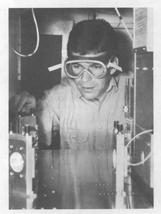
SCOTT BISSON (8354) adjusts the internal optics of a laser light source for a lidar telescope. A Raman lidar sensing device emits timed laser pulses and then measures the backscattering of light that occurs. The backscattered light can be measured to characterize atmospheric content and water vapor densities.
